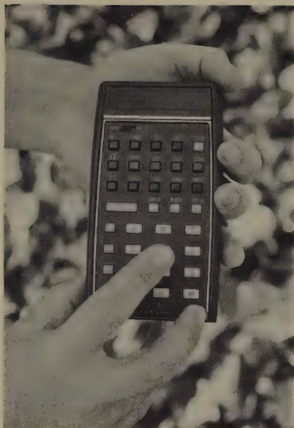
The Hewlett-Packard Pocket Calculator. As of 1974 it is programmable with magnetic cards.
